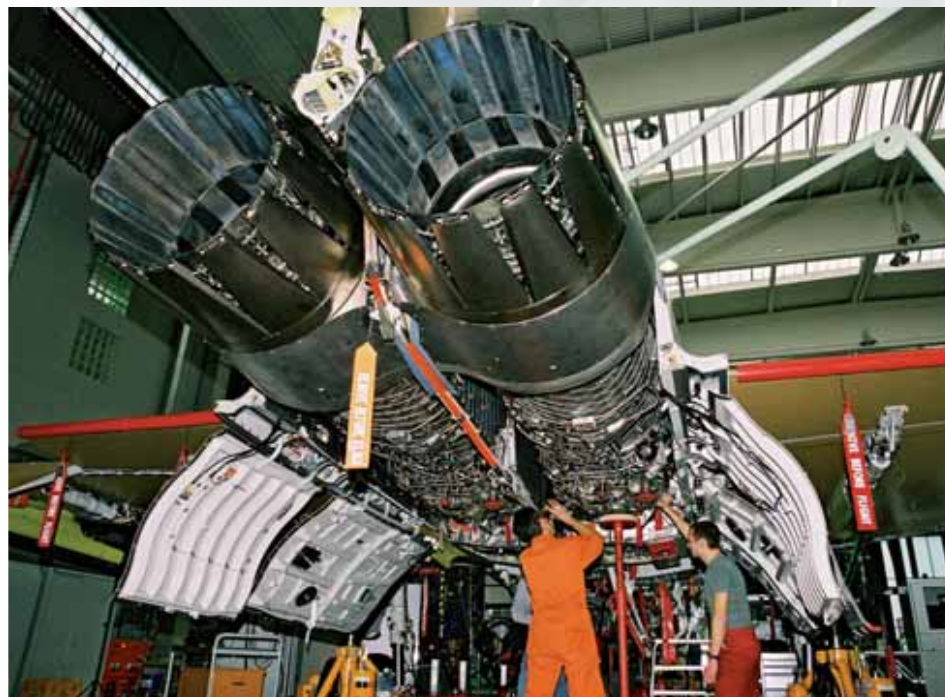
EJ200 installation on Eurofighter Typhoon
