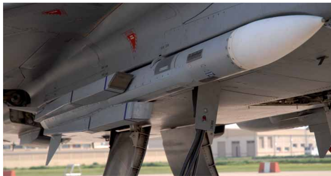
Meteor fitted to the forward eject launch station on Eurofighter Typhoon
