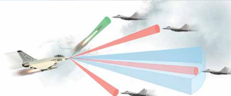
Simultaneous tracking of multiple targets is fulfilled to a higher performance level with an AESA radar
