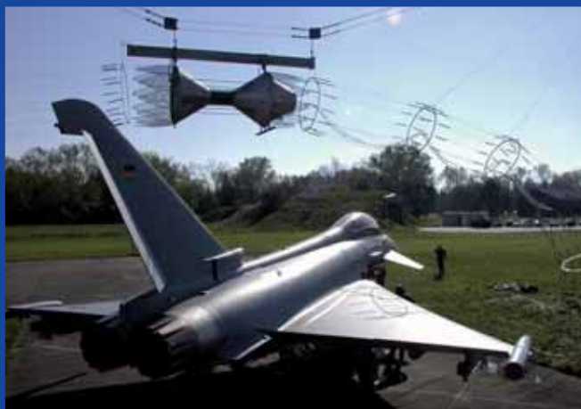
The aircraft will undergo a series of EMP tests
