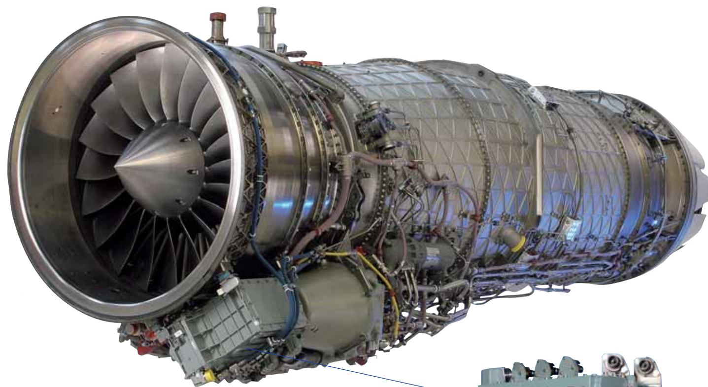
The DECMU is engine-mounted and linked to the aircraft's flight control system
