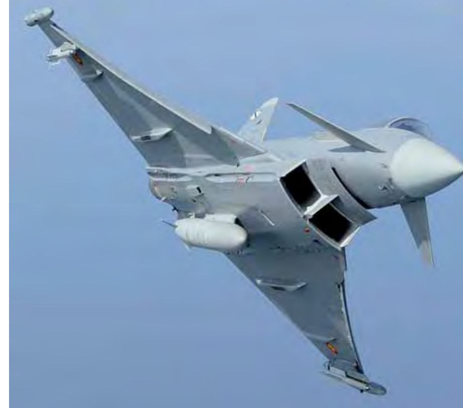
Spanish Eurofighter Typhoon equipped with two IRIS-T missiles and drop tank maneuvering over the Spanish coastline
