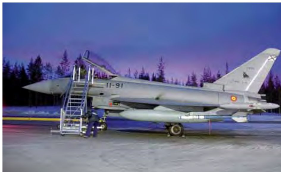
IPA4 undergoing Cold Weather Trials in temperatures as low as -31°C in Vidsele, Sweden.
