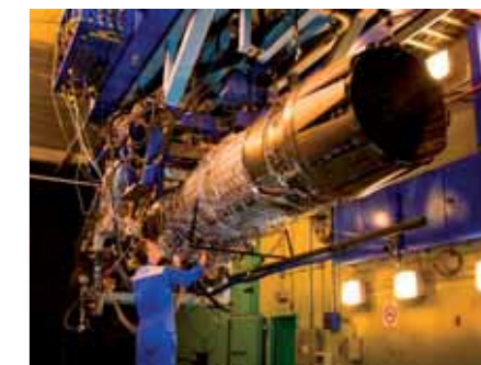
EJ200 engine on the testbed at ITP's facilities
