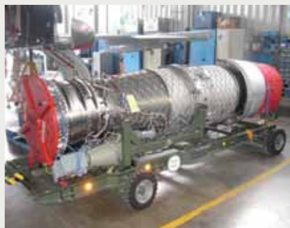
The Tranche 2 EJ200 ready for installation into IPA2
